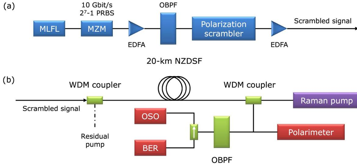
Fig. 2. (Color online) Experimental setup: (a) 10 Gb/s RZ transmitter; (b) all-optical polarization attraction block. MLFL, mode-locked fiber laser; MZM, Mach-Zehnder modulator.
