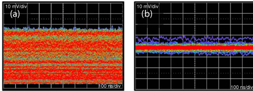
Fig. 4. (Color online) Intensity profile (detected behind a polarizer) of the output CW signal, without (a) and with (b) the 850 mW counterpropagating Raman pump wave. The signal power at the input of the fiber was fixed to 250 mW.
