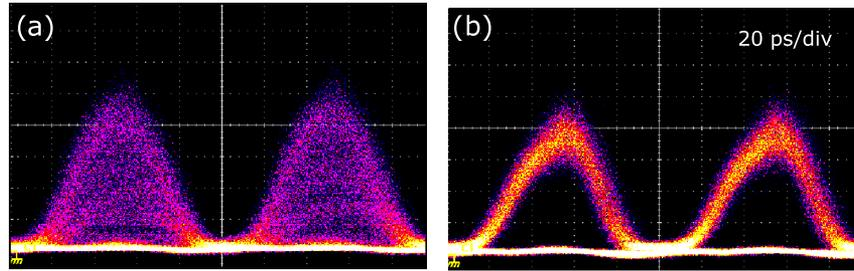
Fig. 7. (Color online) Eye-diagram (detected behind a polarizer) of the output 10 Gbit/s, without (a) and with (b) the counterpropagating Raman pump wave. Signal and pump average power were fixed to 24 dBm (250 mW) and 850 mW, respectively.
