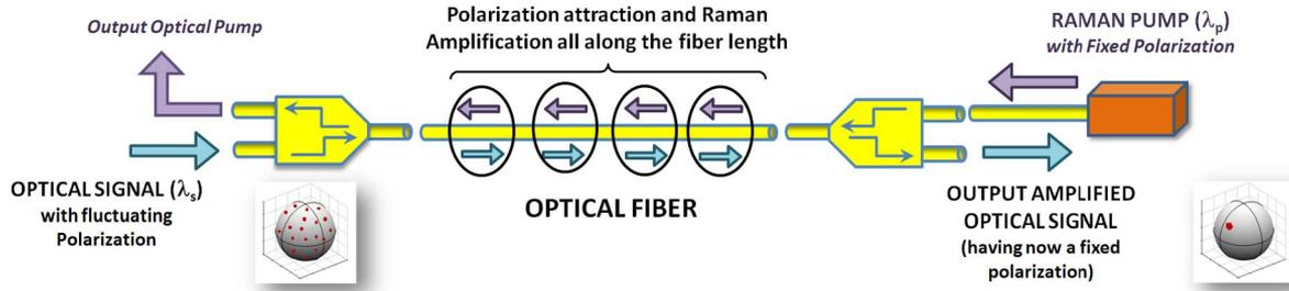
Fig. 1. (Color online) Principle of the device allowing both polarization attraction and Raman amplification.
