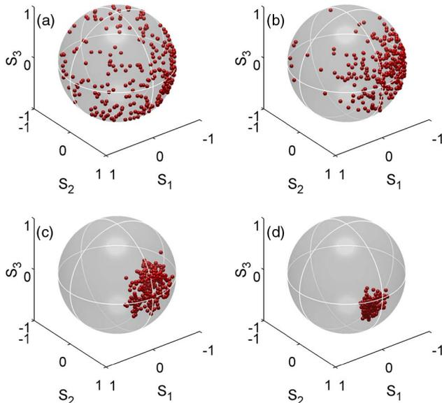
Fig. 5. (Color online) Evolution of the SOP of the 10 Gbit/s signal wave at the output of the fiber as a function of Raman pump power. (a) 0 mW; (b) 200 mW; (c) 400 mW, and (d) 850 mW. The signal power was fixed to 24 dBm. A 6.7 dB on/off gain was achieved for a pump power of 850 mW.
