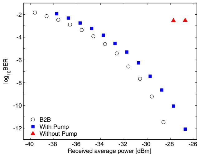
Fig. 8. (Color online) Evolution of the BER as a function of average power in back-to-back configuration (circles); at the output of the system, with polarization scrambling and after a polarizer with (squares) and without (triangles) the 850 mW counterpropagating pump beam.
