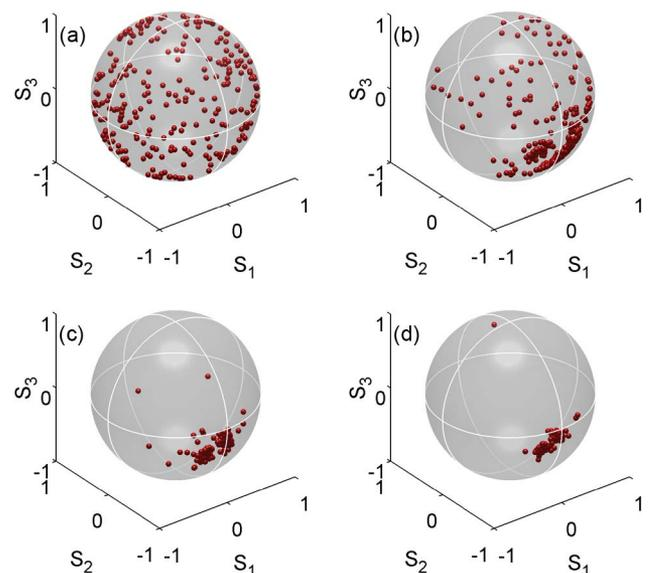
Fig. 3. (Color online) Evolution of the SOP of the output cw signal as a function of the Raman pump power. (a) 0 mW; (b) 340 mW; (c) 680 mW, and (d) 850 mW. The signal power was fixed to 250 mW.
