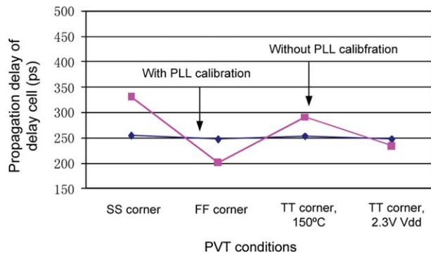
**Figure 6** Simulated delay of the proposed delay cell with and without PLL calibration. [Color figure can be viewed in the online issue, which is available at [wileyonlinelibrary.com](http://wileyonlinelibrary.com)]
