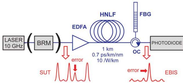
**Figure 1** Experimental set-up. [Color figure can be viewed in the online issue, which is available at [wileyonlinelibrary.com](http://wileyonlinelibrary.com)]
