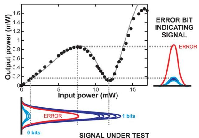
**Figure 2** Transfer function of the proposed device. Experimental results (black circles, results obtained at a repetition rate of 10 Gbps) are compared with the numerical predictions based on the nonlinear Schrödinger equation (solid grey line). [Color figure can be viewed in the online issue, which is available at [wileyonlinelibrary.com](http://wileyonlinelibrary.com)]
