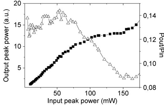
Fig. 2. Output peak power and transmission function  $P_{\text{out}}/P_{\text{in}}$  of the power limiter at 170 Gb/s as a function of the input peak power.
