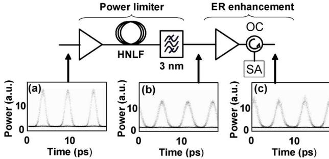
Fig. 4. Regenerator setup.
