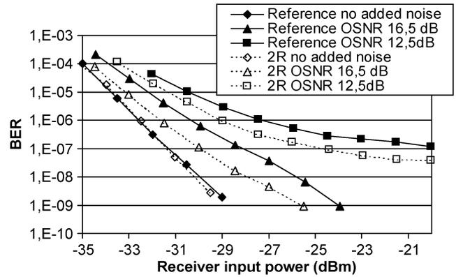
Fig. 5. Receiver sensitivity with and without the regenerator.
