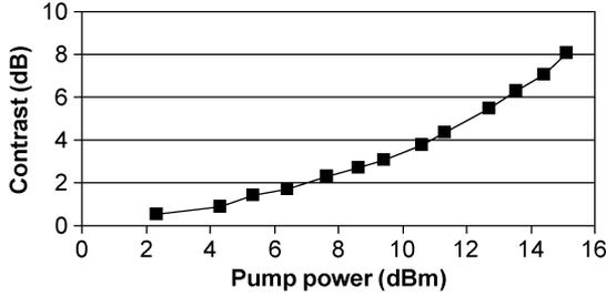
Fig. 1. SA contrast versus pump power at 170 Gb/s.
