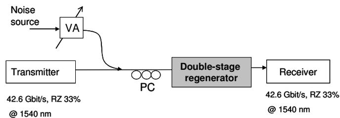
Fig. 7. Experiment setup for back-to-back characterizations. VA: variable attenuator; PC: polarization controller.
