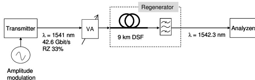
Fig. 1. Setup for the nonlinear interaction experiments. VA: variable attenuator; DSF: dispersion-shifted fiber.
