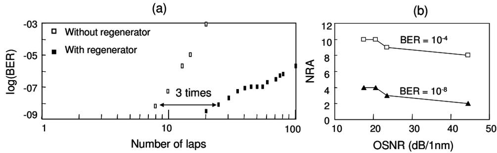
Fig. 11. (a) Evolution of BER as a function of laps in the loop, OSNR = 23.5 dB/1nm, 1 lap = 10 km; (b) Noise resistance assessment as a function of the OSNR for different output BER.
