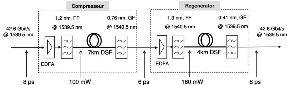
Fig. 6. Experimental setup for the proposed wavelength-transparent double-stage regenerator. FF: Flat-top filter; GF: Gaussian filter; EDFA: Erbium doped fiber amplifier; DSF: dispersion-shifted fiber.
