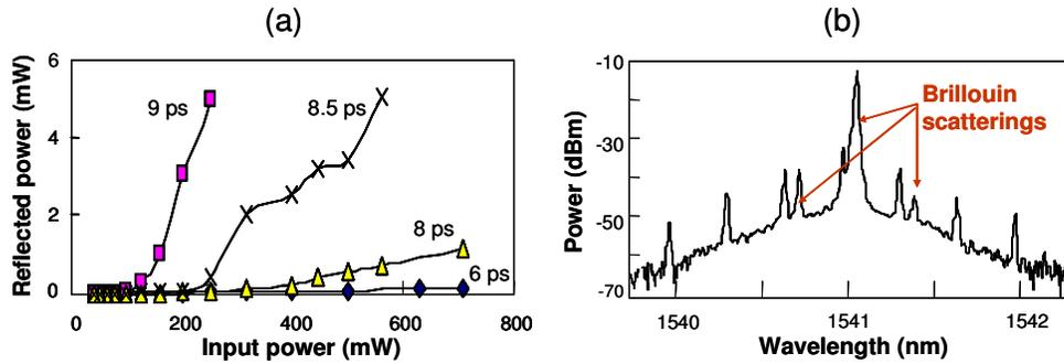
Fig. 5. (a) Evolution of the reflected power as a function of input power in the 4-km long DSF fiber for 4 different input pulse widths; (b) Spectrum of the reflected signal for a pulse width of 8.5 ps with an input power of 300 mW.
