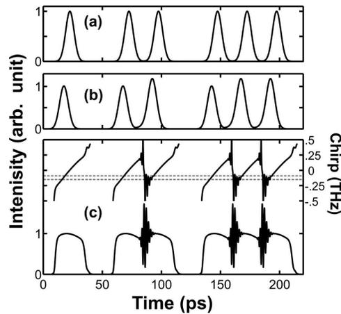
Fig. 3. Numerical simulation results. (a) Input signal; (b) Regenerator output signal for an input average power of 450 mW; (c) Intensity and chirp profiles of the pulses after propagation in the DSF fiber and before spectral filtering.
