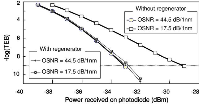
Fig. 8. BER evolution as a function of the power received on the photodiode.
