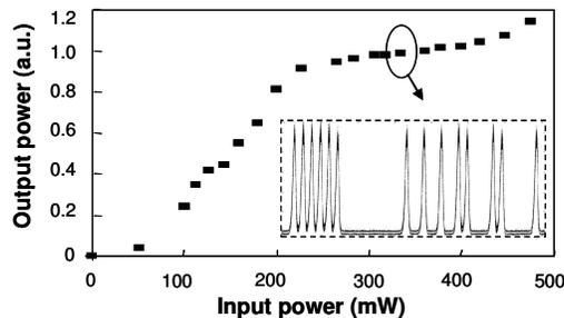
Fig. 4. Experimental transfer function of the regenerator for a 4-km long DSF and 6-ps input pulse width produced from the compressor. Inset shows the experimental data sequence at optimum power (320 mW).
