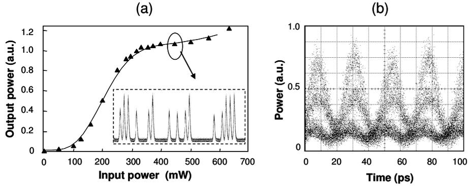
Fig. 2. (a) Experimental (triangles) and theoretical (solid line) transfer functions of the regenerator. Inset: output optical data stream for a working average power of 450 mW; (b) Eye diagram of the regenerator output signal for a working power of 450 mW.
