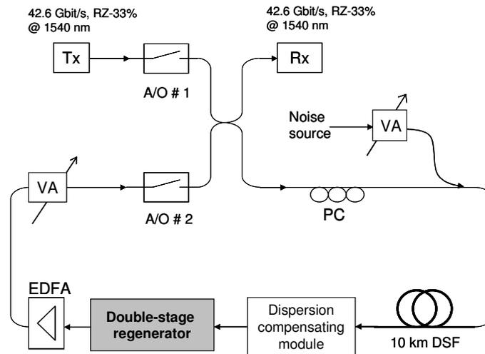
Fig. 10. Experimental setup of the short recirculation loop. Tx: Transmitter; Rx: Receiver; A/O: Accouter optical switch; PC: polarazation controller; VA: variable attenuator; DSF: dispersion shifted fiber; EDFA: Erbium doped fiber amplifier.
