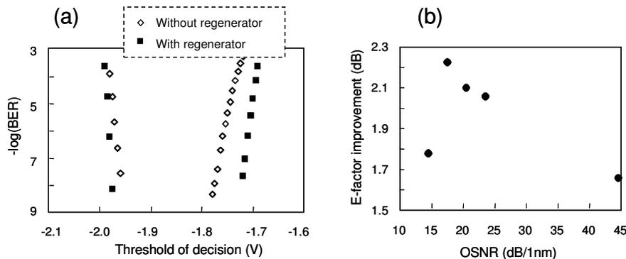
Fig. 9. (a) BER evolution as a function of the decision threshold for an OSNR of 17.5 dB/1nm; (b) Eye-opening improvement as a function of the OSNR.
