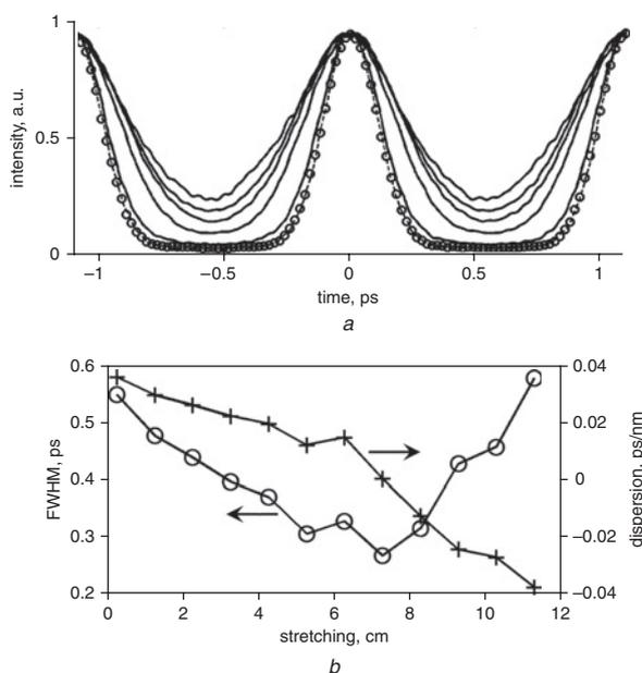
Fig. 2 Autocorrelation function and FWHM of 640 GHz pulse train
