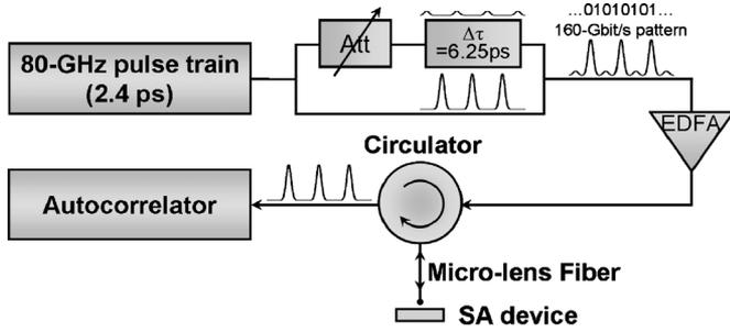
Fig. 1. Experimental setup. Att: variable optical attenuator.  $\Delta\tau$ : delay line. EDFA: erbium-doped fiber amplifier.
