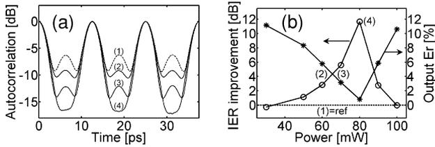
Fig. 2. (a) Autocorrelation functions of the 160-Gb/s pattern as a function of the SA input average power. (1) SA input reference. (2) 60 mW (17.8 dBm). (3) 70 mW (18.5 dBm). (4) 80 mW (19 dBm). (b) Intensity extinction ratio improvement (circles) and ratio of energy  $E_r$  contained in the ghost-pulses at the SA output (stars) as a function of the input average power.
