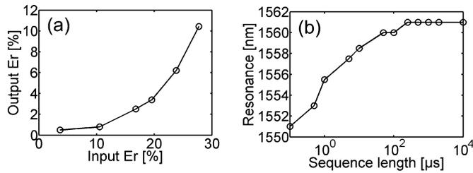
Fig. 4. (a) Nonlinear response of our SA device: ratio of energy  $E_r$  contained in the ghost-pulses at the output of the SA device as a function of the input ratio. (b) Resonance wavelength as a function of the sequence length.
