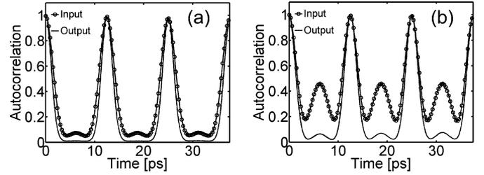
Fig. 3. Autocorrelation functions of the 160-Gb/s sequence at the input (circles) and output (solid lines) of the SA device. (a) In:  $E_r = 3.7\%$ ; out:  $E_r = 0.5\%$ . (b) In:  $E_r = 19.6\%$ ; out:  $E_r = 3.4\%$ , respectively.
