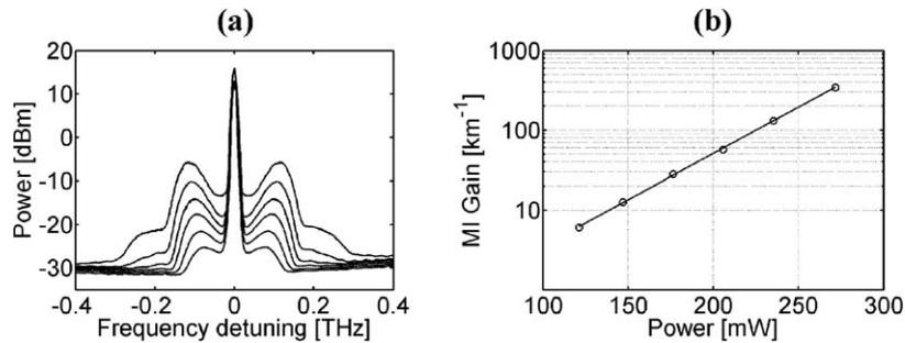
Fig. 3. (a) Evolution of the MI sidebands at 1550 nm as a function of input power, from bottom to top,  $P = 120, 145, 175, 205, 235,$  and  $270$  mW. (b) Evolution of MI gain as a function of input power, measurements (circles) and linear fit (solid line).
