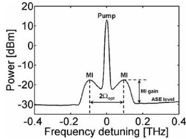
Fig. 2. Experimental MI spectrum obtained for a pump power of 200 mW at 1549.9 nm.
