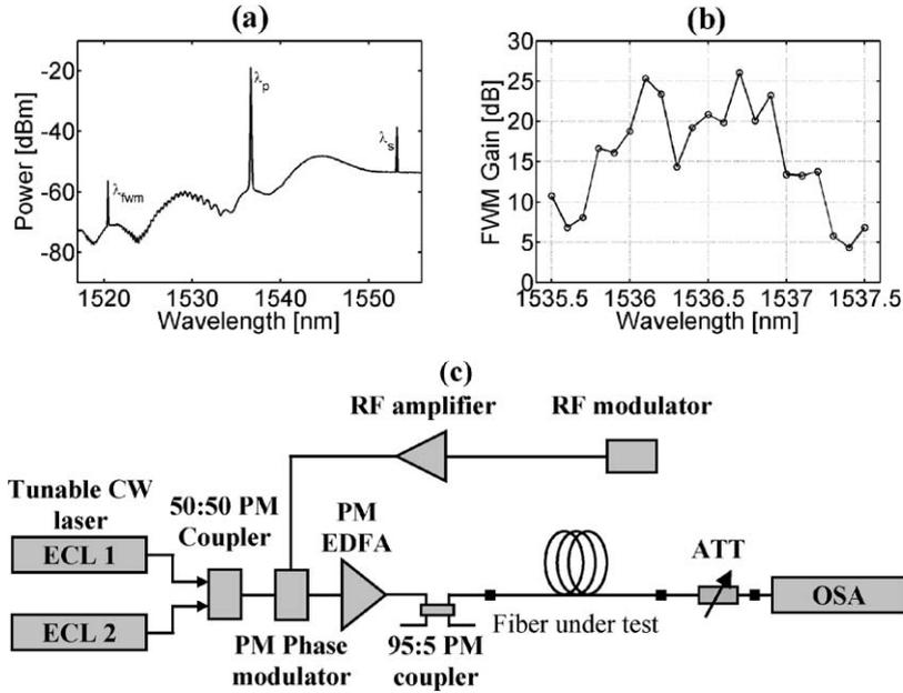
Fig. 5. (a) Spectrum of the FWM process when the pump wavelength is near the zero dispersion.  $\lambda_p = 1536.7$  nm,  $P_p = 80$  mW,  $\lambda_s = 1532$  nm, and  $P_s < 1$  mW. (b) FWM efficiency as a function of pump wavelength near the zero dispersion. (c) Experimental setup of the zero-dispersion measurement technique.
