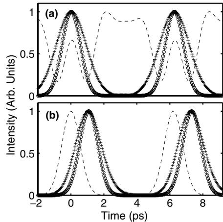
Fig. 2. (a) Pulse train at the fiber output for  $\Omega = 160$  GHz (solid line),  $\Omega = 160.001$  GHz (circles),  $\Omega = 160.01$  GHz (crosses) and  $\Omega = 160.1$  GHz (dashed line). The fiber length is  $L = L_{\beta_3} = 511L_{\beta_2}$ . (b) Pulse train at the fiber output for  $\Omega = 160$  GHz (solid line),  $\Omega = 160.1$  GHz (circles),  $\Omega = 161$  GHz (crosses). Dashed line: pulse train at the fiber input. The fiber length is  $L = L_{\beta_3}/6 = 4L_{\beta_2}$ .
