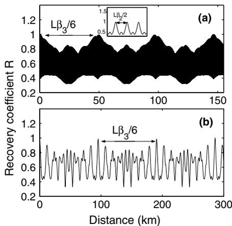
Fig. 1. Evolution of the recovery coefficient  $R(z)$  with the distance. (a)  $L_{\beta_3}/6 = 48.8$  km and  $L_{\beta_2}/2 = 287.5$  m. The inset represents a zoom around  $z = L_{\beta_3}/6$ . (b)  $L_{\beta_3}/6 = 95.3$  km and  $L_{\beta_2}/2 = 11.9$  km.
