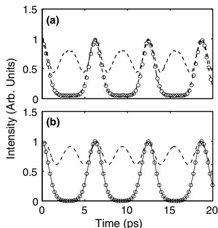
Fig. 4. (a) Plot showing the experimental autocorrelation traces of the pulse train measured at the fiber output for  $\Omega = 160$  GHz (circles) and  $\Omega = 164$  GHz (dashed line), in comparison with those measured at the fiber input for  $\Omega = 160$  GHz (solid line). (b) Plot showing the corresponding theoretical autocorrelation traces.
