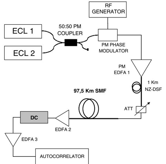
Fig. 3. Experimental set-up. ECL 1, ECL 2: external-cavity lasers; PM: polarization-maintaining; EDFA: erbium-doped fiber amplifier; ATT: variable attenuator; DC: dispersion compensator module.
