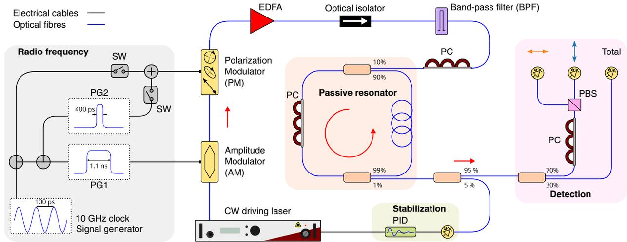
FIG. 2. Experimental setup. The passive fiber ring resonator is highlighted with an orange background. PG1 and PG2, pattern generators; SW, electrical switch; EDFA, erbium-doped fiber amplifier; PC, polarization controller; PBS, polarizing beam splitter.
